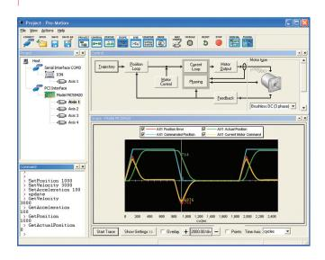
Pro-Motion is a sophisticated, easy-to-use Windows-based exerciser program for use with the ATLAS Digital Amplifiers, ION Digital Drives and other PMD motion control ICs and cards.
